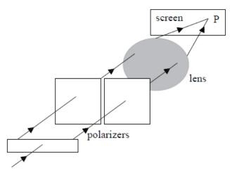
A lens brings the light to focus at point P on a screen. The lens does not introduce any additional path difference.
