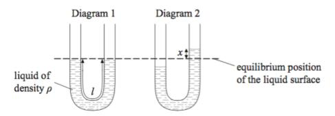
The pressure on the liquid in one side of the tube is increased so that the liquid is displaced as shown in diagram 2. When the pressure is suddenly released the liquid oscillates. The damping of the oscillations is small.
