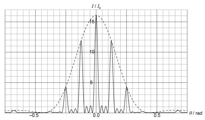
$I_0$  is the intensity of the light at the middle of the screen from **one** slit.
