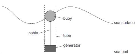
The motion of the buoy can be assumed to be simple harmonic.
