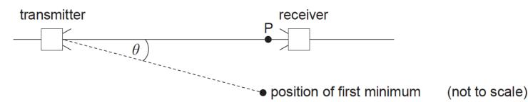
The microwaves emerge from the transmitter through an aperture that acts as a single slit.
